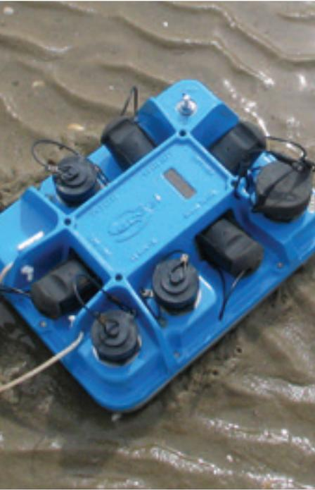
*The LAUX is used to connect each line in a 3D spread to the higher speed transverse connection to the recording system.*
